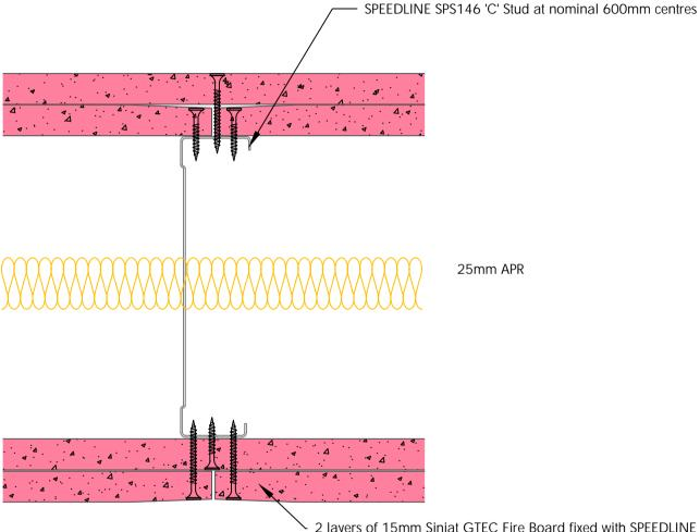
2 layers of 15mm Siniat GTEC Fire Board fixed with SPEEDLINE Drywall Screws at 300mm centres (200mm centres at external angles). Ref to table for fixing length.
